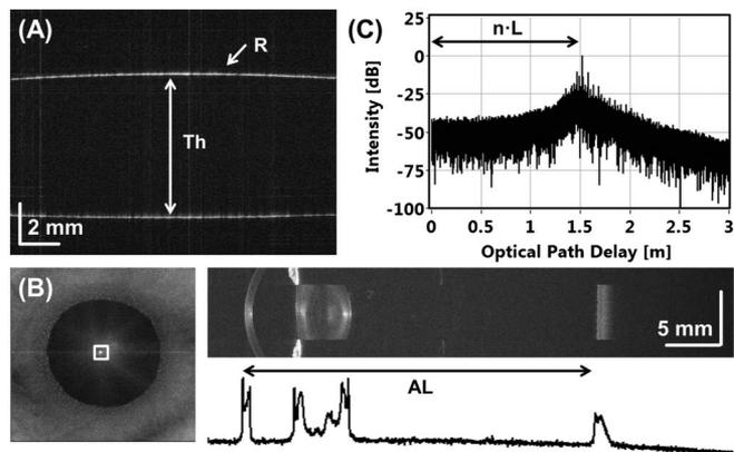
Fig. 2. Long-range SS-OCT imaging and quantitative measurement. (A) Cross-sectional image of a cylindrical lens enables measurement of central thickness  $Th$  and radius  $R$  of the surface curvature. (B) Full eye length imaging enables accurate determination of axial eye length  $AL$  (ocular biometry). (C) MZI measurement of optical fiber length  $L$  ( $n = 1.4696$ ).
