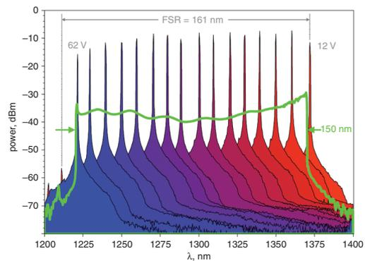
**Fig. 3** Static and dynamic tuning response of our ultra-widely tunable MEMS-VCSELs
