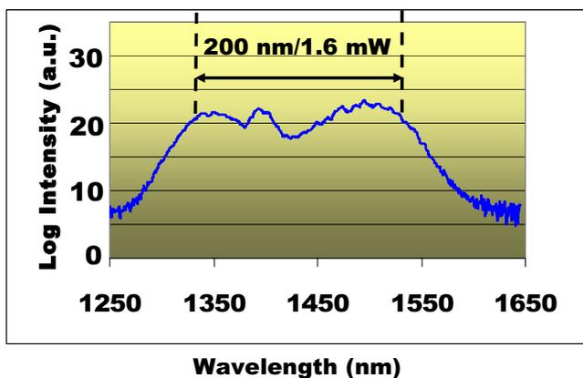
Figure 8: Combined spectrum when SLDs of Fig. 7 are combined through device of Fig. 6. The possibility of still wider bandwidth remains, if the full width of the individual SLDs can be realized. The low intensity in the center of the spectrum could be eliminated by better centering of the two spectra, and this should allow future devices with  $>200$ nm 3dB bandwidth.
