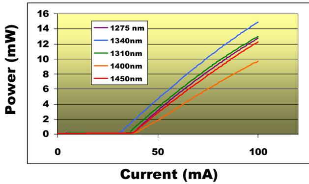
Figure 4: L-I curves associated with each of 5 laser channels, with wavelengths shown in legend.
