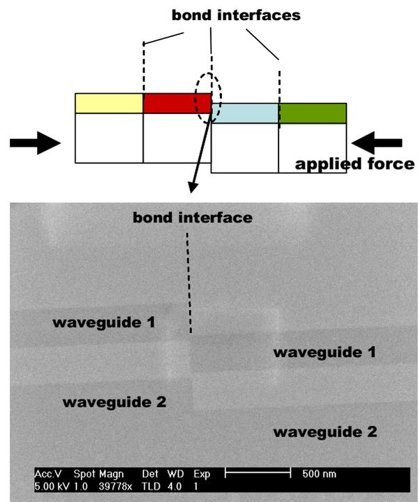
**Figure 1:** Geometry of multi-lateral wafer bonding. Vertical misalignment highlights the bonded interface.
