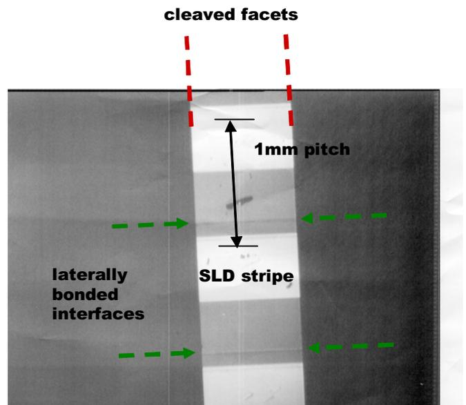
Figure 3: Photograph of laterally bonded coarse wavelength division multiplexer (CWDM) laser array, illustrating smooth continuous cleaved facets across lateral bonds.
