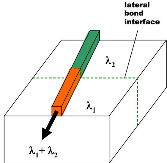
Figure 6: Two section superluminescent diode (SLD) in which the waveguide straddles the bonded interface. Spectral bands from two different gain regions ( $\lambda_1$  and  $\lambda_2$ ) are generated within a common waveguide, and the output represents, to first order, a superposition of the two spectra.
