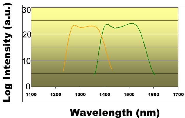
Figure 7: Two superluminescent diode (SLD) gain regions and associated spectra before combining in device of Fig. 6. Each SLD has approximately 100 nm bandwidth.
