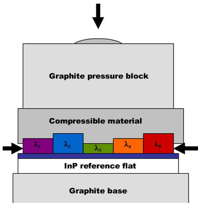
Figure 2: Minimization of vertical misalignments during lateral bonding, enabling low-loss waveguide junctions.
