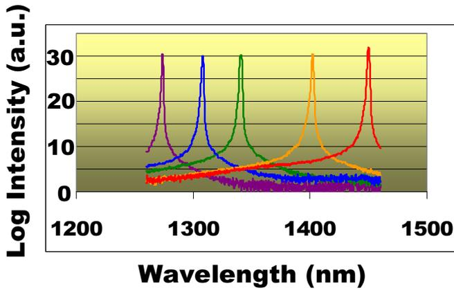
Figure 5: Laser Spectra of coarse wavelength division multiplexer (CWDM) array with 180 nm span.
